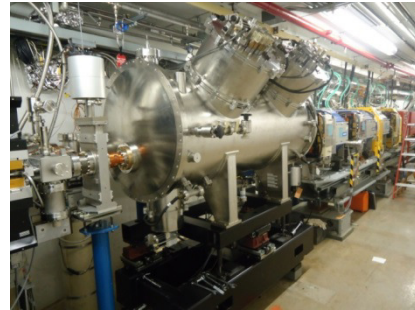
Figure 1: SCU0 installed in the APS storage ring.
