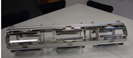
Figure 3: Electrostatic LEBT quadrupole triplet assembly. The length of the assembly is 91 cm.
