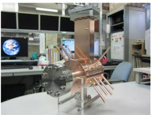
Figure 6: Manufactured ECC RF gun.
