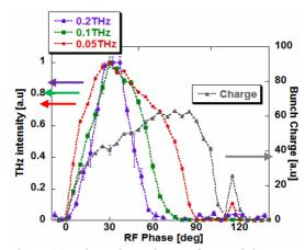
Figure 11: Phase dependence of several detectors.
