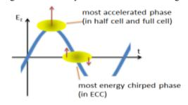
Figure 2: Off-crest acceleration in ECC.
