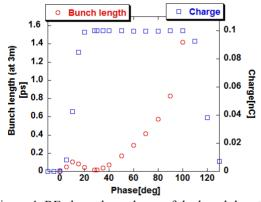
Figure 4: RF phase dependence of the bunch length.
