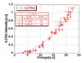
Figure 10: 0.2 THz coherent synchrotron radiation.
