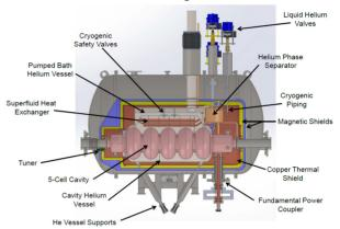
Figure 1: Lavout of the 704 MHz SRF cryomodule.
