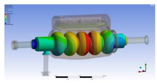
Figure 7: Deformed shape of the 5-cell cavity.
