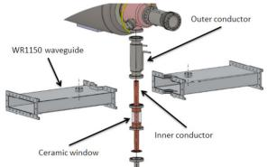
Figure 3: Fundamental power coupler model.
