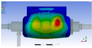
Figure 6: Deformed shape of the helium vessel.
