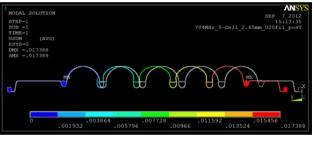
Figure 5: Relaxed and deformed shapes of the cavity.
