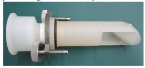
Figure 2: Single injection quill used for FRIB  $\beta$ =0.53 HWR cavity BCP processing.
