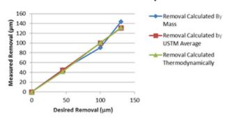
Figure 5: Comparison of measurement techniques for each stage of  $\beta$ =0.53 cavity bulk etch.
