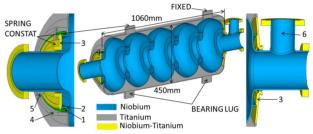
Figure 6: COMSOL model of mechanical assembly used in simulations. 1–bellows, 2–stiffening ring between end half-cell and conical flange, 3–conical flange, 4–bellows ring, 5–support brackets, 6–main coupler. Left – tuner end group. Right – main coupler end group.
