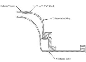
Figure 3: He vessel to cavity sliding joint design.
