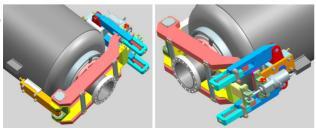
Figure 5: Lever tuner installed on dressed 5 cell cavity.
