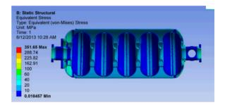
Figure 9: Equivalent Stress distribution at 2 K with 4 bar pressure applied.
