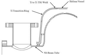
Figure 2: He vessel to cavity fixed joint design.
