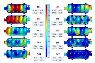
Figure 8: Frequencies, total energy, and COMSOL plots of normalized displacements of 10 lowest mechanical modes. Normalization is 1 mm maximum displacement.
