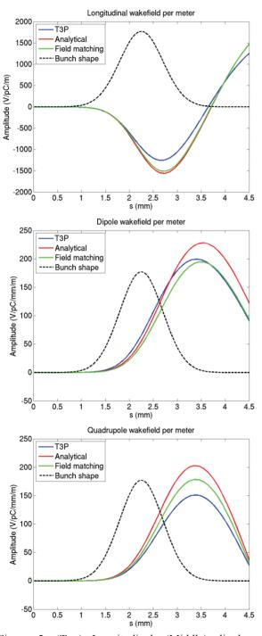
Figure 5: (Top) Longitudinal, (Middle) dipole, and (Bottom) quadrupole wakefield per meter length of the dechirper obtained by the analytical, field matching and numerical approaches.
