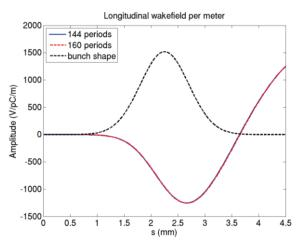
Figure 4: Longitudinal wakefield per unit length of the dechirper with 144 and 166 corrugations.
