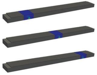
Figure 3: Snapshots of beam transit in the dechirper with 160 corrugation periods. The beam comes in from the left boundary at the origin (the lowest corner) and moves to the right. The colored region in each snapshot indicates the moving window at the corresponding time.
