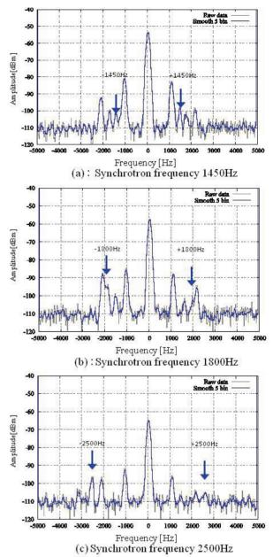
Figure 5: Frequency spectra when RF voltage was varied. RF frequency 2.5MHz is at the centre (0Hz). Synchrotron frequencies are indicated by blue arrows. Unexplainable low peaks were observed at  $\pm 1.7$ kHz in (a) and  $\pm 1.5$ kHz in (b). They were not noises. Those low peaks were not observed under no beam.
