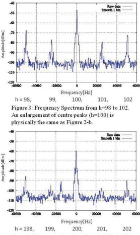
Figure 4: Frequency Spectrum from h=198 to 202. The peak between 199 and 200 is a noise since it was observed under no beam.
