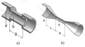
Figure 1: a) Step Collimator. b) Tapered Collimator.
