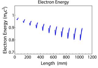
Figure 8: Electron energy distribution of the train of bunches as they travel through the structure. The bunches are injected at an energy of 500 keV (0.98 m<sub>e</sub>c<sup>2</sup>).
