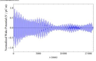
Figure 5: Longitudinal wake potential as a function of the distance behind the impulse bunch (s).
