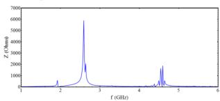
Figure 6: Longitudinal wake impedance shown as a function of frequency.
