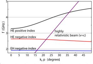
Figure 3: Dispersion curves of TM modes in the metamaterial waveguide. Two modes exist that couple to the electron beam, a negative refractive index mode at 2.5-2.6 GHz (red) and a positive index mode at 3.5-4.5 GHz (black). The relativistic electron beam dispersion line is also shown  $(2\pi f = k_z c$ , purple).
