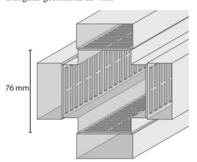
Figure 1: Metamaterial waveguide assembled from four WR187 waveguides (47.55 x 22.15 mm) with CSRRs machined into inner face of assembled structure.
