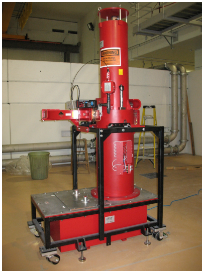
Figure 2: CPI type VKL7967A 1.3 GHz cw klystron
