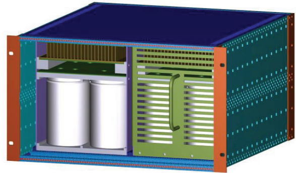
Figure 7: A single 19" rack with 2 RFPAs modules arrangement scheme.
