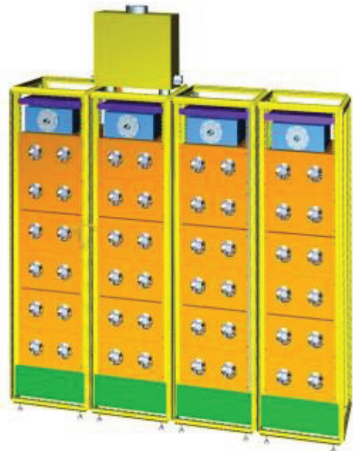
Figure 6: A row of 4 19" cabinets with common output power combiner.
