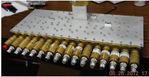
Figure 4: High power 16-to-1 combiner cold test.
