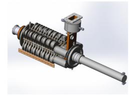
Figure 1: The 10 kW CW S-Band PPM Klystron.
