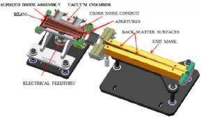
Figure 2: XBPM 2 design. A pair of apertures and four Si PIN diodes form a pinhole camera to read out the position of the x-ray footprint on the exit mask.
