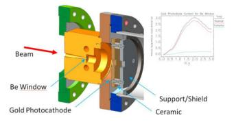
Figure 3: IM2 uses Rayleigh- and Compton-scattered x-rays from the Be window to monitor the x-ray beam intensity. Inset: A photodiode is used to detect x-rays.
