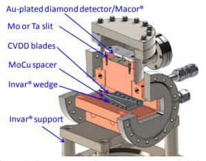
Figure 6: Compton-scattering XBPM conceptual design for the APS canted undulator front end.
