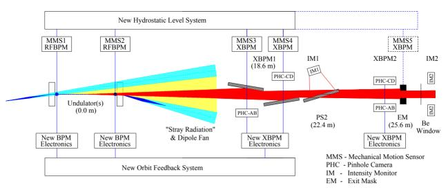
Figure 5: In the APS-U orbit feedback system, the XBPM system is responsible for measuring the x-ray beam angle and monitoring the x-ray beam intensity and position outside of the feedback loop.
