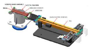
Figure 4: IM1 uses Cu K-edge XRF to measure the x-ray beam intensity when the photon shutter is closed.
