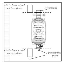
Figure 1: Custom SS end-groups assembled onto cavity during vertical testing.
