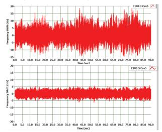
Figure 2: Microphonic detuning - Original design (top), redesigned (bottom) cavity/tuner system.
