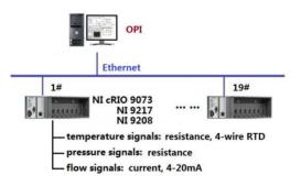
Figure 3: Hardware structure of the HLS Cooling Water Monitor System.
