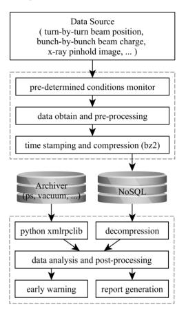
Figure 1: The architecture of data logging system.
