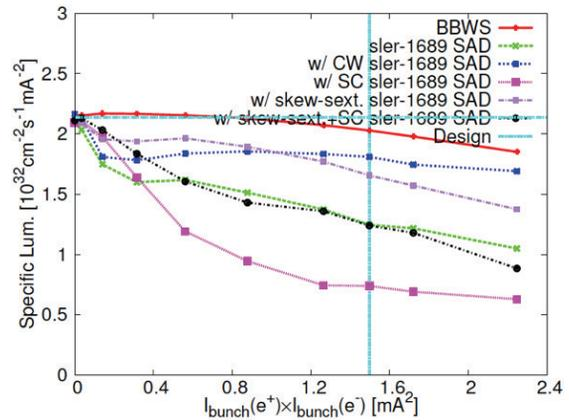
Figure 7: Luminosity can be partially recovered by inserting a skew sextupole map into LER of SuperKEKB.
