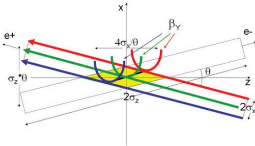
Figure 1: Crab-waist collision scheme. The color straight lines show directions of motion for particles with different horizontal deviations from the central orbit. The arrows indicate the corresponding  $\beta$  function variations along these trajectories.
