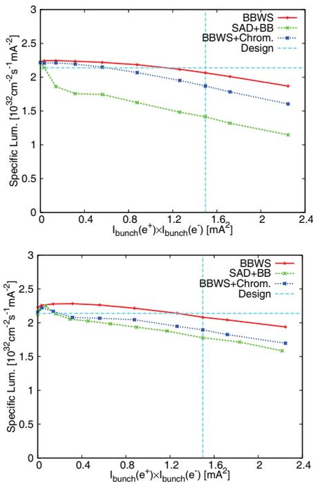
Figure 5: Specific luminosity as a function of bunch current products at SuperKEKB. Top picture is for LER, and bottom picture is for HER.
