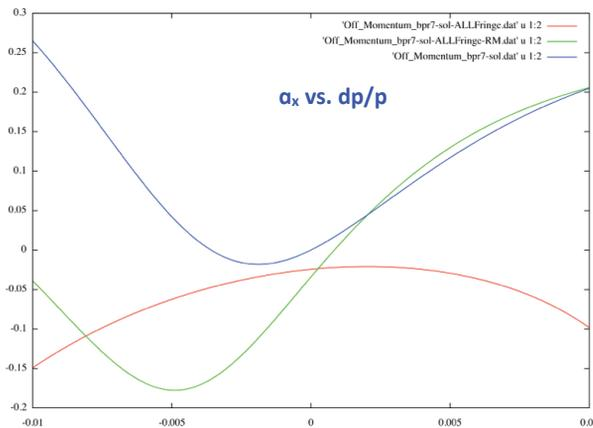
Figure 8: The  $\alpha_x$  versus  $\delta$  at IP for original hard-edge(blue)/soft-edge(red) model and corrected(green) soft-edge model.
