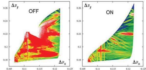
Figure 3: Beam-beam footprint with crab sextupoles off (left) and on (right) obtained by FMA techniques [7]
