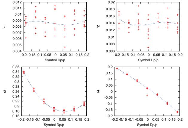
Figure 4: Measurement of the chromaticity for x-y coupling in KEKB-LER.
