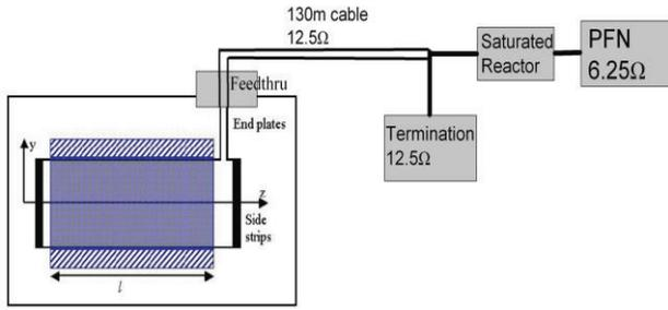
Figure 1: The schematic view of kicker system.
