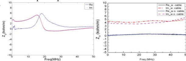
Figure 5: Transverse impedance by wire-loop method.
