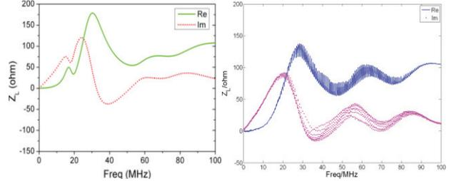
Figure 2: Longitudinal impedance by coaxial-method (left: without connection with cable and PFN; right: connection with the cable and PFN).
