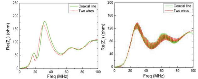
Figure 3: Longitudinal impedance by twin-wire method (left: without connection with cable and PFN; right: connection with the cable and PFN).
