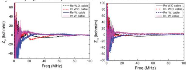
Figure 4: Transverse impedance by twin-wire method.
