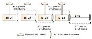
Figure 3: The RF driving and FCT on linac.
