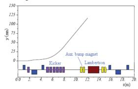
Figure 4: The layout of extraction system with bump magnets.
