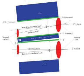
Figure 6: Schematic diagram of the Lambertson septum magnet cross section along the beam.
