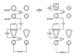
Figure 2: Schematic map of accelerator for the high current ion source.
