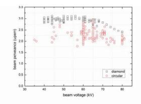
Figure 4: Beam perveance as a function of beam voltage with different type of plasma grids.
