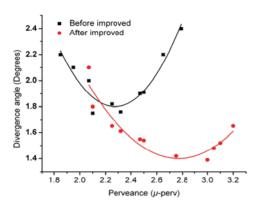
Figure 5: Divergence angle as a function of perveance with circular and diamond grids.
