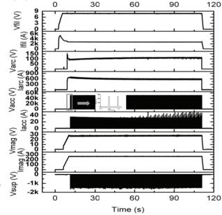
Figure 6: Long pulse ion beam extraction of 100s with beam energy of 50 keV and beam curent of 33 A.
