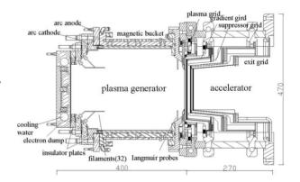
Figure 1: Schematic of high current ion source.
