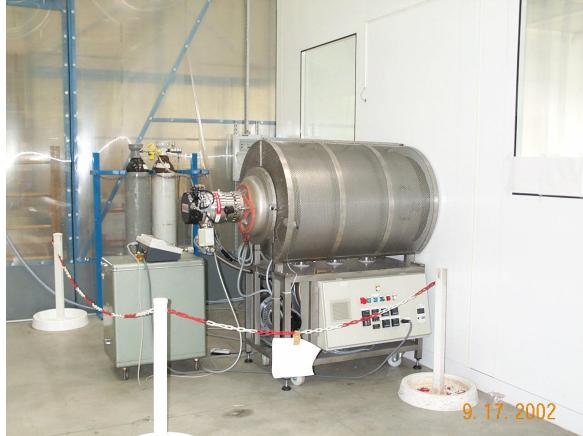
Figure 1: The vacuum furnace connected to the wall of the class 10 clean room area.
