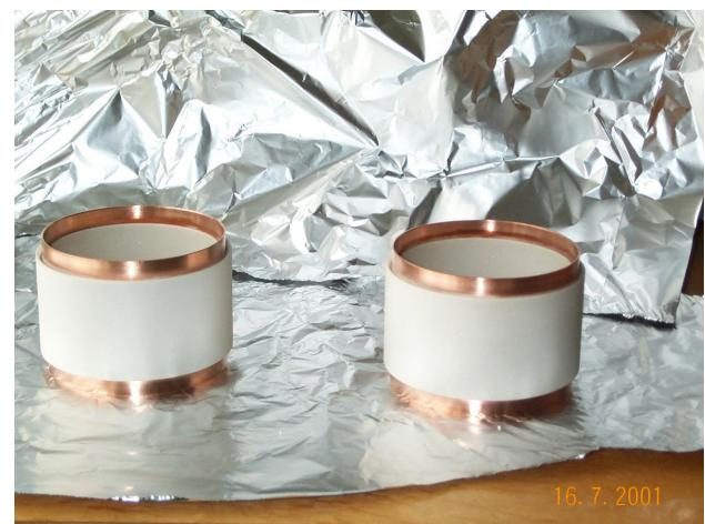
Figure 3: TTF-IV coupler ceramic windows brazed to their copper collars.
