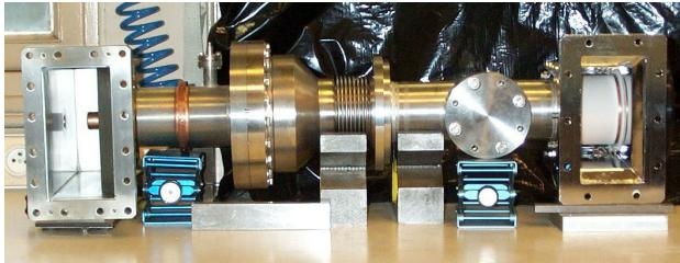
Figure 4: TTF-IV coupler attached to wave-guide test box. The warm window is to the right of the photograph.
