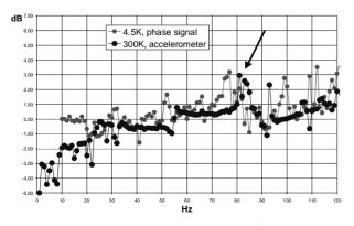
Figure 1: Mechanical response of the  $\beta$ =0.7 cavity to longitudinal excitation: the main resonance, pointed by the arrow, is around 77 Hz at 4.5K (81 at 300K).
