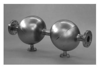
Figure 3: PACO, the 633 mm long superconducting resonator for the detection of gravitational waves.
