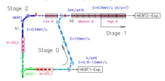
Figure 1: Stages 0, 1 and 2 for the ISAC-II upgrade.
