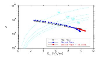
Figure 2: RF cold test results comparing cavity performance with a flat tuner plate and the new slotted plate.
