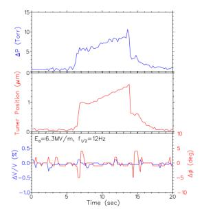
Figure 3: Tuner response to forced helium pressure flucuation ( $\frac{\Delta f}{\Delta P}=1$ Hz/Torr) and corresponding voltage (blue) and phase (red) errors for high field ( $E_a$ =6.3 MV/m) and a bandwidth of  $\pm 12$  Hz.
