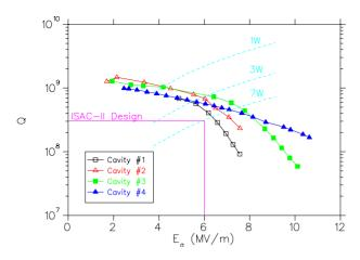
Figure 4: Cold test results for the cavities of the first medium beta cryomodule.
