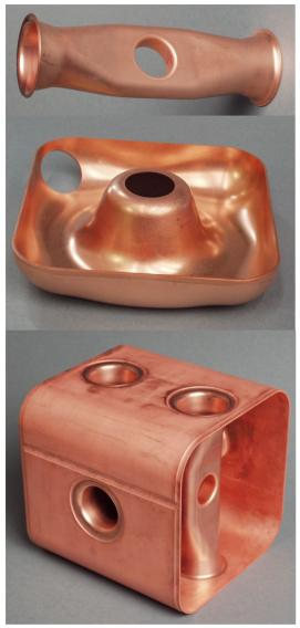
Figure 10: FZJ triple-spoke cavity copper model.
