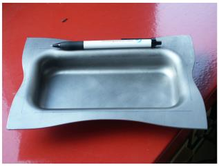
Figure 5: High pressure hydroforming of 230x160x2mm3 niobium sheet, depth: 30mm, 10mm bending radius.
