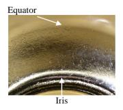
Figure 7a: Picture of the inner surface of C1-10 (residual Q-slope after baking).
