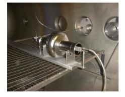
Figure 3: Internal view of plasma reactor with cavity, permanent magnets and gas inlet system.
