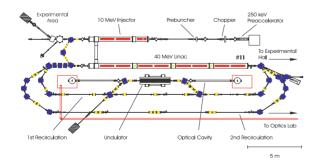
Figure 1: Layout of the S-DALINAC
