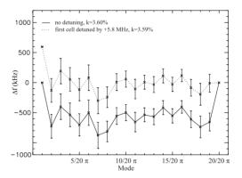
Figure 6: Difference between the measured passband frequencies and the calculated frequencies in case of a flat field profile (solid line) and in case of a perturbed field profile resulting from a detuned edge cell (dashed line).
