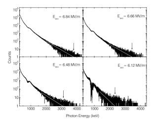
Figure 4: Bremsstrahlung spectra measured with a BGO detector for different accelerating gradients.
