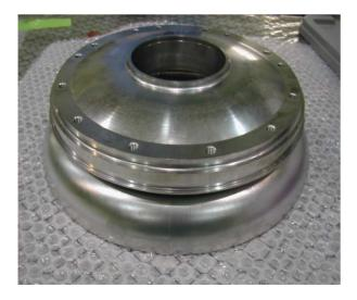
Figure 4: An end-cell with a titanium endplate.
