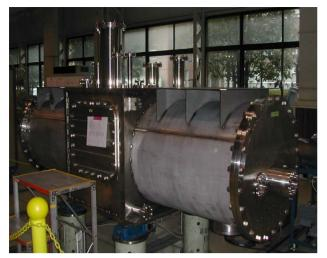
Figure 2: Vacuum vessel.
