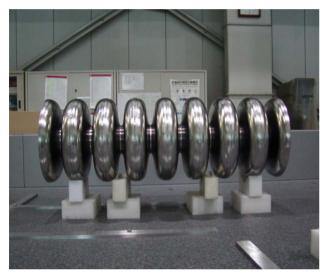
Figure 3: A welded center-cells.
