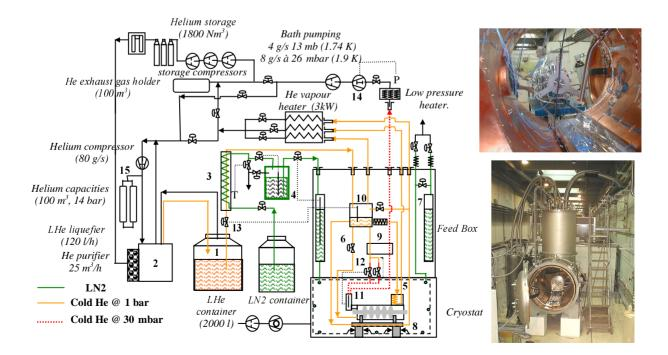
Figure 3: Cryogenic Installation.
