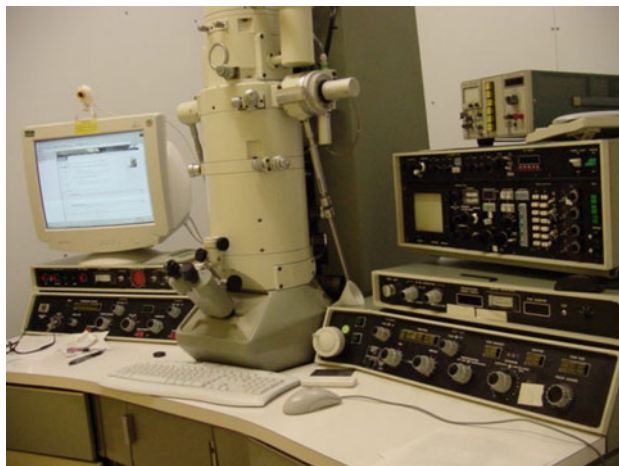
Fig.3: Transmission electron microscope and scanning transmission electron microscope.
