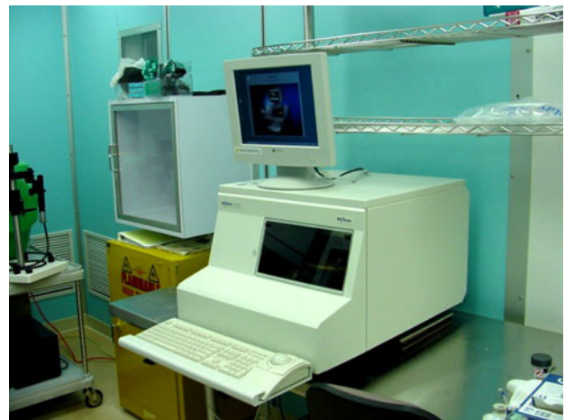
Fig.7: 3-dimension large scan area profilometer with a vertical resolution as high as 0.1 nm
