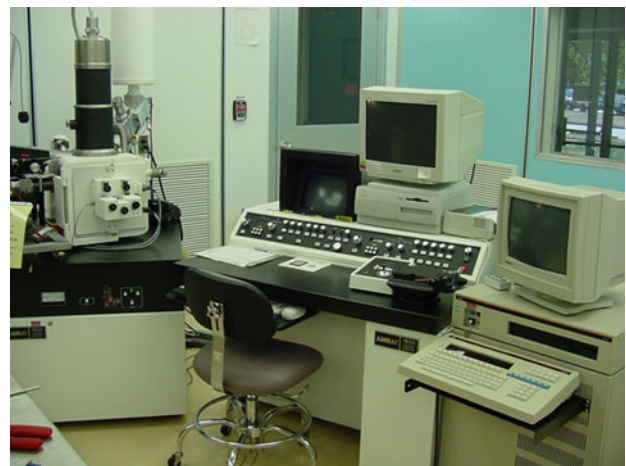
Fig.2 Scanning electron microscope equipped with energy dispersive x-ray analysis.
