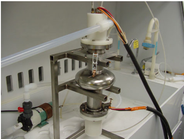
Fig.17: One of the setups for electroplishing on Nb single cell cavities.
