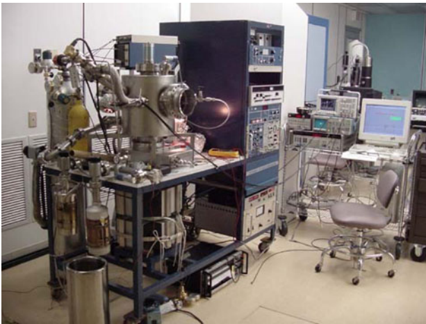
Fig.5: Home-made secondary ion mass spectrometry.
