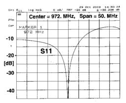
Figure 4: Measured S-parameter (reflected power) in the high power test stand.
