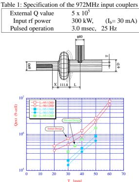
Figure 1: Model cavity and the calculated external Q.
