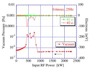
Figure 10: Vacuum pressure and electron activities after processed up to 2.2 MW.
