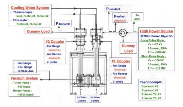
Figure 6: Experimental instrumentation for high power tests.
