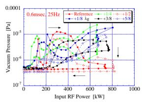
Figure 11: Rf processing in the standing wave.
