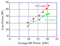
Figure 13: Rf loss at the rf window and the inner conductor.
