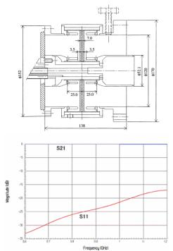
Figure 2: Drawing of a 972MHz coaxial ceramic window and the calculated S-parameters.
