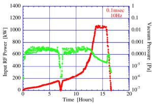
Figure 7: Rf processing logs in the initial test.
