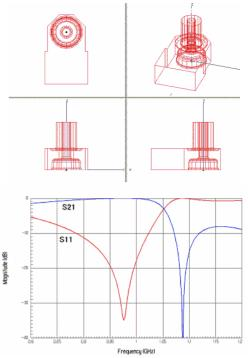
Figure 3: Designed structure of a 972MHz doorknob and the calculated S-parameters.
