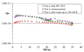
Figure 3: Behaviour of the cavity AC76 after warm up to 120-140 C and cool down again.
