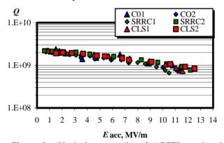
Figure 8: Vertical test results of ACCEL produced cavities.
