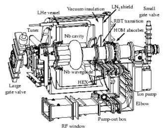
Figure 1: Cornell B-cell cryomodule.
