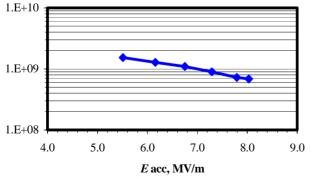
Figure 9: Q vs.  $E_{\rm acc}$  of CLS cryomodule #1. (Courtesy of M. Pekeler, ACCEL.)
