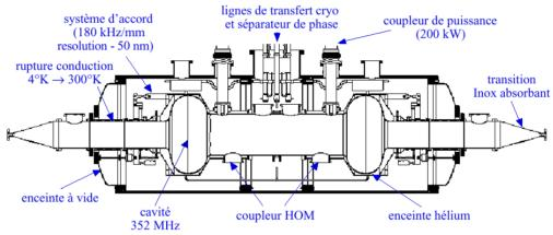
Figure 6: SOLEIL cryomodule [30].
