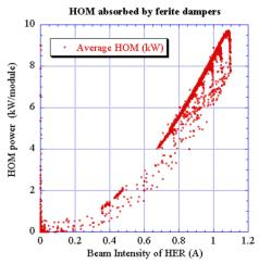
Figure 5: HOM power in KEKB SC cavity. (Courtesy of T. Furuya, KEK.)
