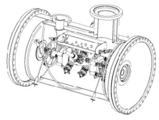
Figure 10: 3D view of the S3HC cryomodule [37].
