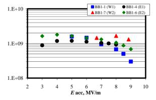
Figure 3: Q vs.  $E_{acc}$  for CESR cavities.
