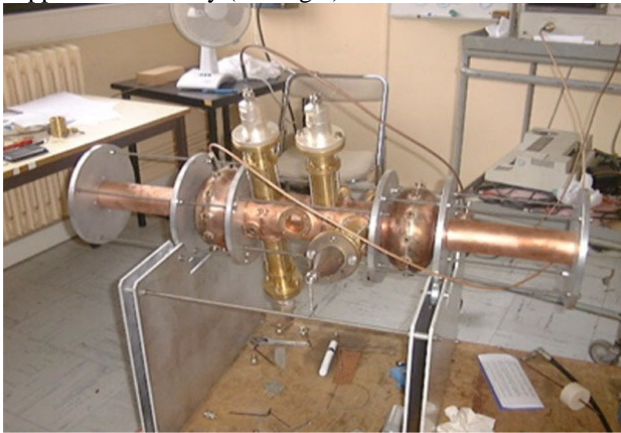
Figure 1: Model cavity for HOMs damping optimisation.
