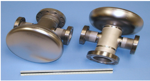
Figure 2: Photograph of the BNL/AES all-niobium half cell cavity.
