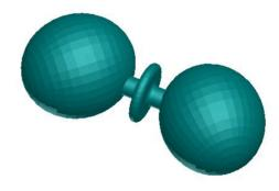
Figure 1: Artistic view of the coupled spherical cavities with the central tuning cell
