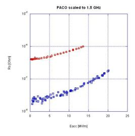
Figure 9: Surface Resistance of the single-cell spherical cavity
