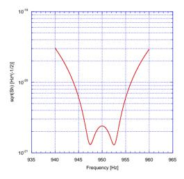
Figure 12: Calculated system sensitivity ( $\omega_m \sim \omega_2 - \omega_1 \sim 1$  kHz,  $\mathcal{Q}=10^{10},\ Q_m=10^6,\ T=1.8$  K,  $T_{eq}=1$  K, stored energy  $U\sim 1$  J per cavity)
