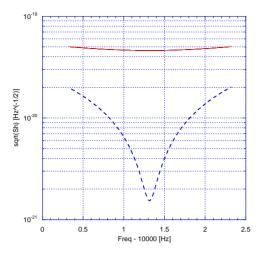
Figure 11: Calculated system sensitivity ( $\omega_m \sim 4$  kHz,  $\omega_2 - \omega_1 \sim 10$  kHz,  $\mathcal{Q} = 10^{10}$ , T = 1.8 K,  $T_{eq} = 1$  K, stored energy  $U \sim 10$  J per cavity and a)  $Q_m = 10^3$  (solid line); b)  $Q_m = 10^6$  (dashed line))
