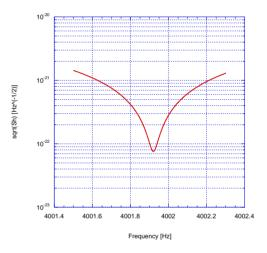
Figure 13: Calculated system sensitivity ( $\omega_m \sim 1 \text{ kHz}$ ,  $\omega_2 - \omega_1 \sim 4 \text{ kHz}$ ,  $\mathcal{Q} = 10^{10}$ ,  $Q_m = 10^6$ , T = 1.8 K,  $T_{eq} = 1 \text{ K}$ , stored energy  $U \sim 1200 \text{ J}$  per cavity)
