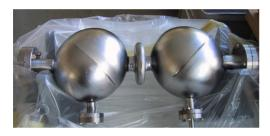
Figure 3: Niobium spherical cavities (variable coupling)
