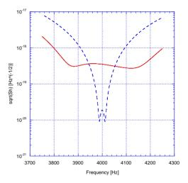
Figure 10: Calculated system sensitivity ( $\omega_m \sim \omega_2 - \omega_1 \sim 4$  kHz,  $\mathcal{Q}=10^{10}$ , T=1.8 K,  $T_{eq}=1$  K, and a)  $Q_m=10^3$ , stored energy  $U\sim 10$  J per cavity (solid line); b)  $Q_m=10^6$ , stored energy  $U\sim 0.1$  J per cavity (dashed line))
