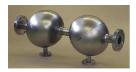
Figure 2: Niobium spherical cavities (fixed coupling)
