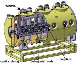
Figure 10: HWR cryomodule.
