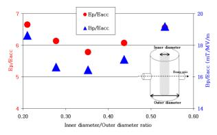
Figure 2: Optimisation of the cavity inner over outer diameter ratio.
