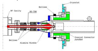
Figure 7: Coupler structure (courtesy of LPSC Grenoble).
