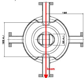
Figure 5: Horizontal cut view of the final HWR prototype in the beam axis region.
