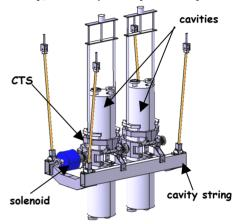
Figure 9: HWR cavity string.
