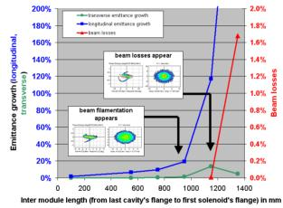
Figure 11: Impact of the inter-module length on the emittance growth and on the beam losses.
