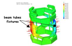
Figure 8: HWR cold tuning system.
