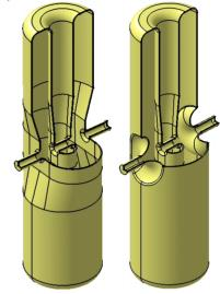
Figure 4: "Juelich-type" (left) and "Argonne-type" (right) HWR models.
