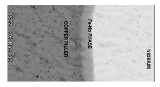
Figure 7: SEM closeup of copper/niobium transition.
