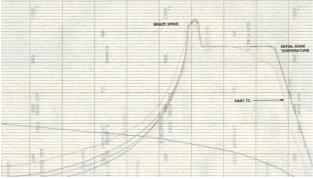
Figure 3: Furnace braze temperature cycle. Time advances from right to left.
