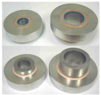
Figure 4: Completed braze assemblies showing (top) joint top surface with braze metal groove and (bottom) joint underside showing fillet.
