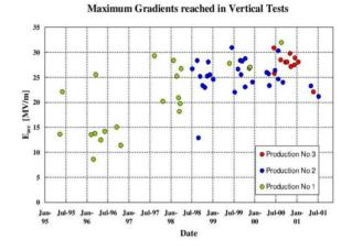
Figure 6: Maximum gradients reached in vertical tests. It is provided by MS EXCEL based on the ASCII file generated by the RGS called from *Summary of Last RF Tests* in the GUI.
