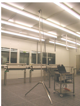
Picture 1: Set up for filter Leak test
