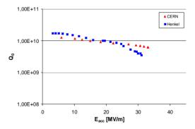
Figure 6: Behaviour of welded cavity after in-situ bake. The CERN test shows good performance of 33 MV/m. The first test after EP at Henkel was suffering from a vacuum leak. The cavity degradation starting at 20 MV/m is due to this problem. The maximum gradient is 31
