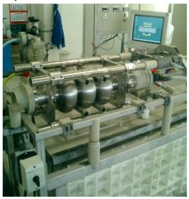
Figure 1: Setup for electropolishing
