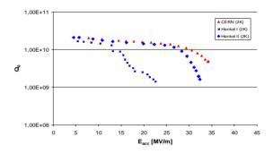
Figure 5: Behaviour of the spun cavity after in-situ bake. The CERN test shows good performance of 35 MV/m. The first test after EP at Henkel was suffering from strong field emission due to problem during the baking preparation at DESY. A new high pressure rinsing improved the performance to fields above 32 MV/m.
