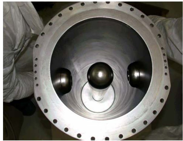
Figure 5: View of Niobium cavity with tuner plate
