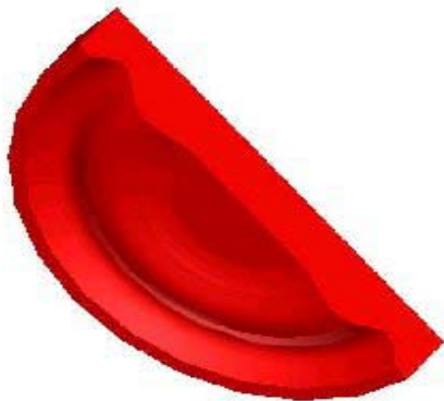
Figure 4: Profile of the tuner plate used in HFSS simulation
