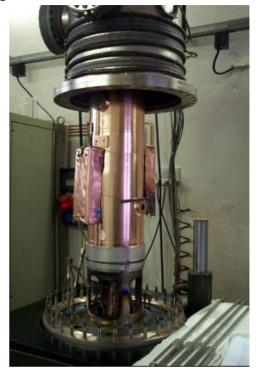
Figure 3: A medium  $\beta$  ALPI cavity mounted in the sputtering chamber.
