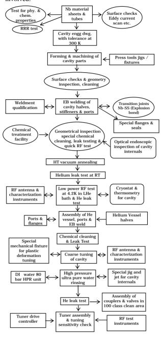
B. Cavity fabrication & stage inspection & testing
