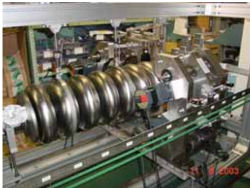
Figure 4: Pre-tuning equipment and a 9-cell Nb cavity
