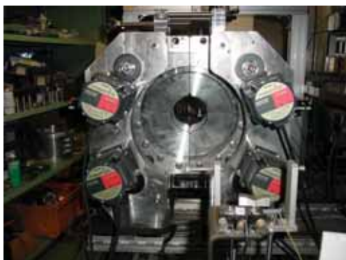
Figure 5: Clamping pads and stepping motors
