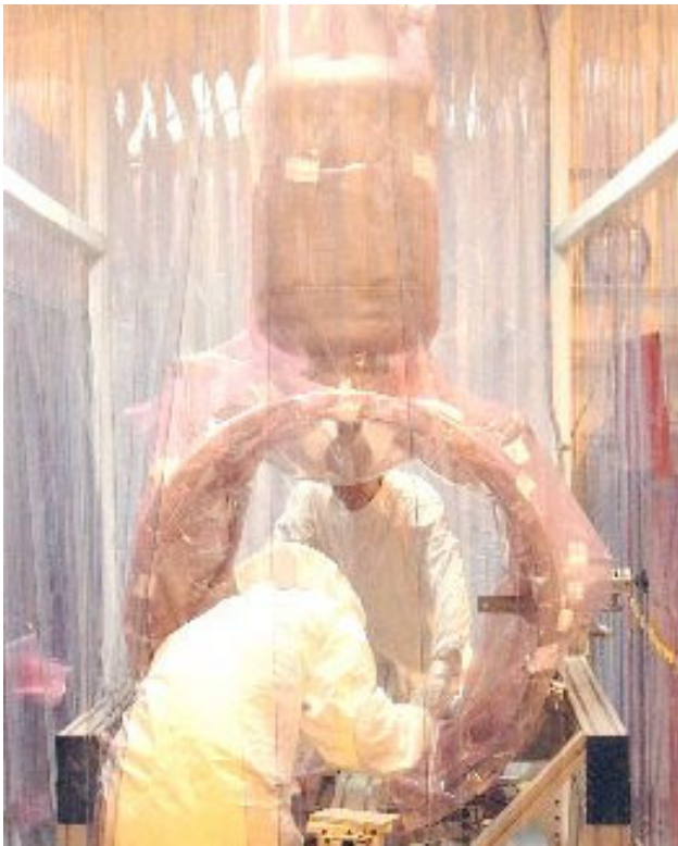
Figure 2. A horizontal test cryostat for the two-cell spoke cavity being moved into a clean assembly area.
