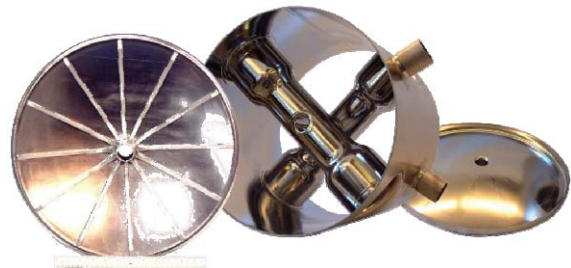
Figure 1. Three pieces of the RIA two-spoke cavity after receiving a heavy electropolish.
