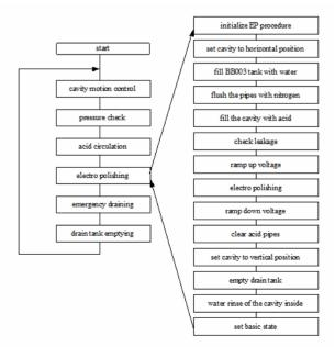
Figure 2: Procedures and sequences of the process [2].
