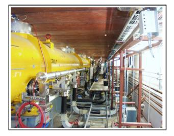
Figure 4: Superconducting TESLA modules installed in the TTF linac during installation of the waveguides.
